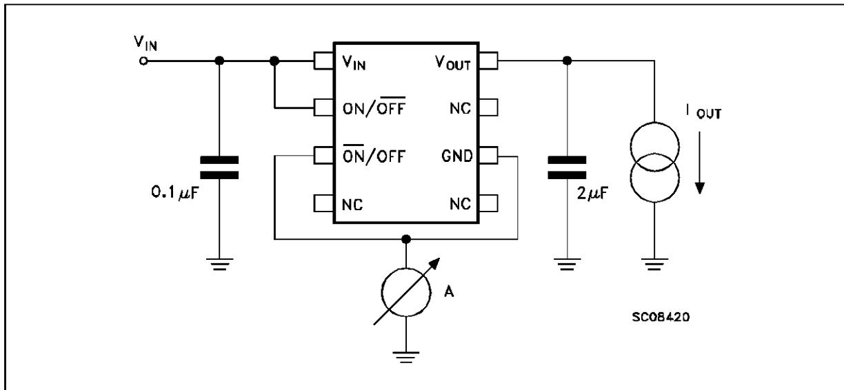
**TEST CIRCUITS:** Supply Current (OFF MODE)
